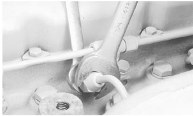
Bleeding Fuel System at Injection Nozzle
