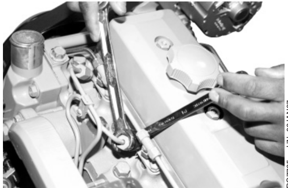
Bleed fuel system at fuel injection nozzles
